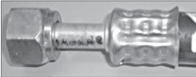
Assembly crimped, rotated and re-crimped.
